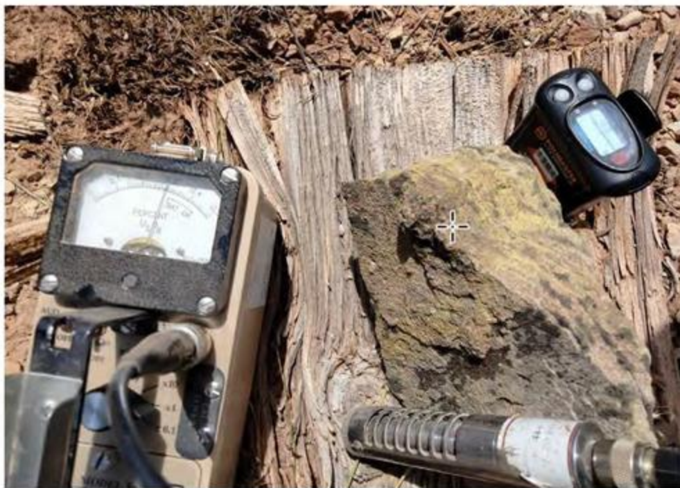
Photo 12.1: Sample 650470 from an unnamed dump on the Fawn claim block. Highly visible carnotite grade 0.3% U_3O_8 in the Ludlum Model 3 Geiger counter. The assay returned 4867 ppm U (0.49% U_3O_8 ) and 3120 ppm V (0.557% V_2O_5 ). Important associated pathfinder metals included 0.5% Ba and 9.4 ppm Mo.
